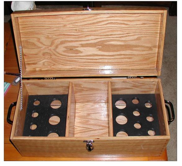
Here's the finished case after eleven coats of urethane on the outside. The inside has five coats. The hardware is heavy chrome intended for marine use.
