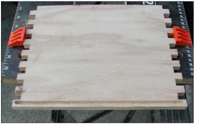
This is one of the ends with a slot for the 'real' base. A false bottom will be glued on to make the bottom smooth.
