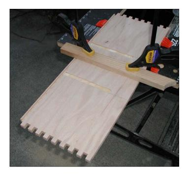
Here's one of the sides with the slots cut in for the two dividers. The Lynn Jig did a great job on the box joints.
